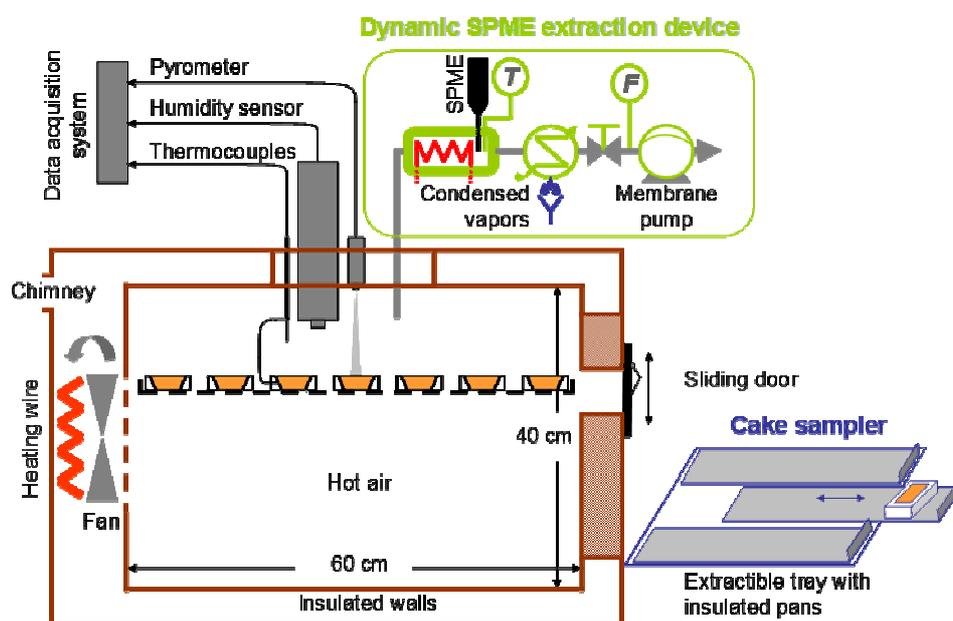
Figure 9: Diagram of the Reactial oven for monitoring the CNFV during cooking. According to the thesis of S. Fehaili (Th1).
