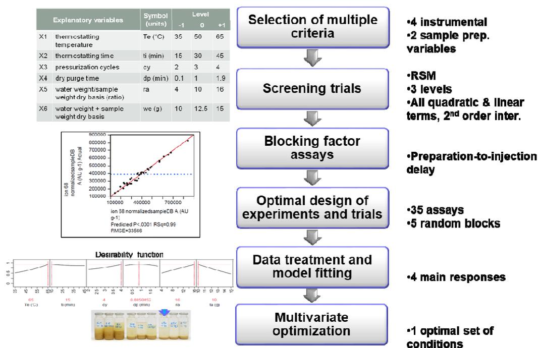
Figure 14: Optimization strategy for the simultaneous quantification of furan and furfural by optimal design of experience and desirability function. Adapted from the thesis of M. Cepeda Vazquez (Th4).
