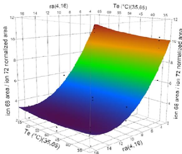
Figure 15: Response area for the ratio furan/d4-furan. Response [ion 68 (furan) area / ion 72 (d4-furan) area] in function of the thermostat temperature (Te) and of the water to sample ratio (ra, dry base). According to ACL5.
