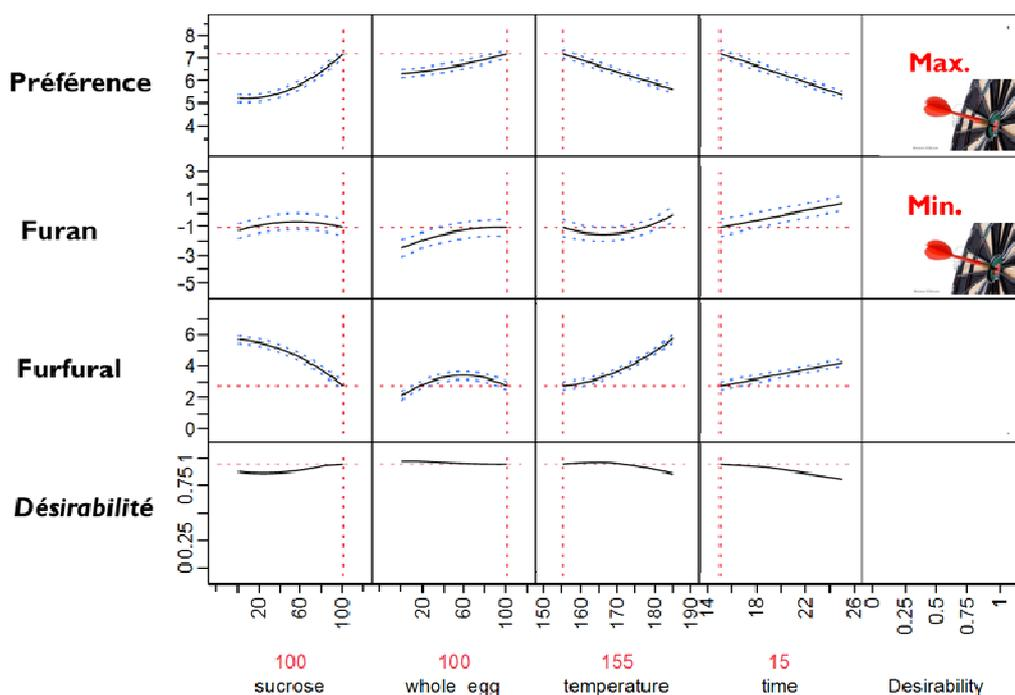
Figure 27: Prediction profilers with the desirability function: decrease in furan and consumer preference (adapted from ACL3).
