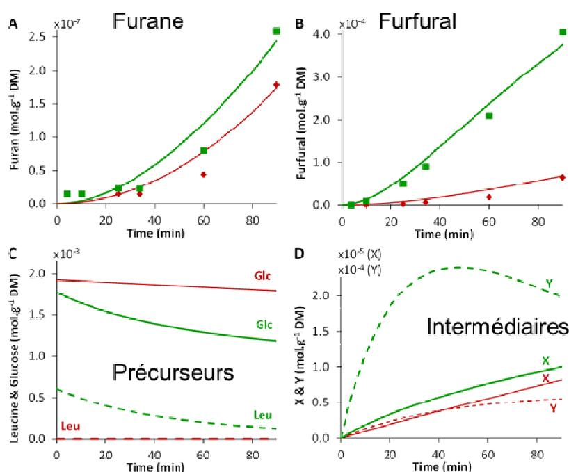
Figure 36: Kinetics of furan and furfural formation generated by cooking at  $170^\circ\text{C}$  in model sponge cakes accompanied by the consumption of precursors and two intermediates. Model G (in red) and model G + L (in green)). The discrete points represent the experimental points and the dotted curves the modeling. Adapted from (ACL4).
