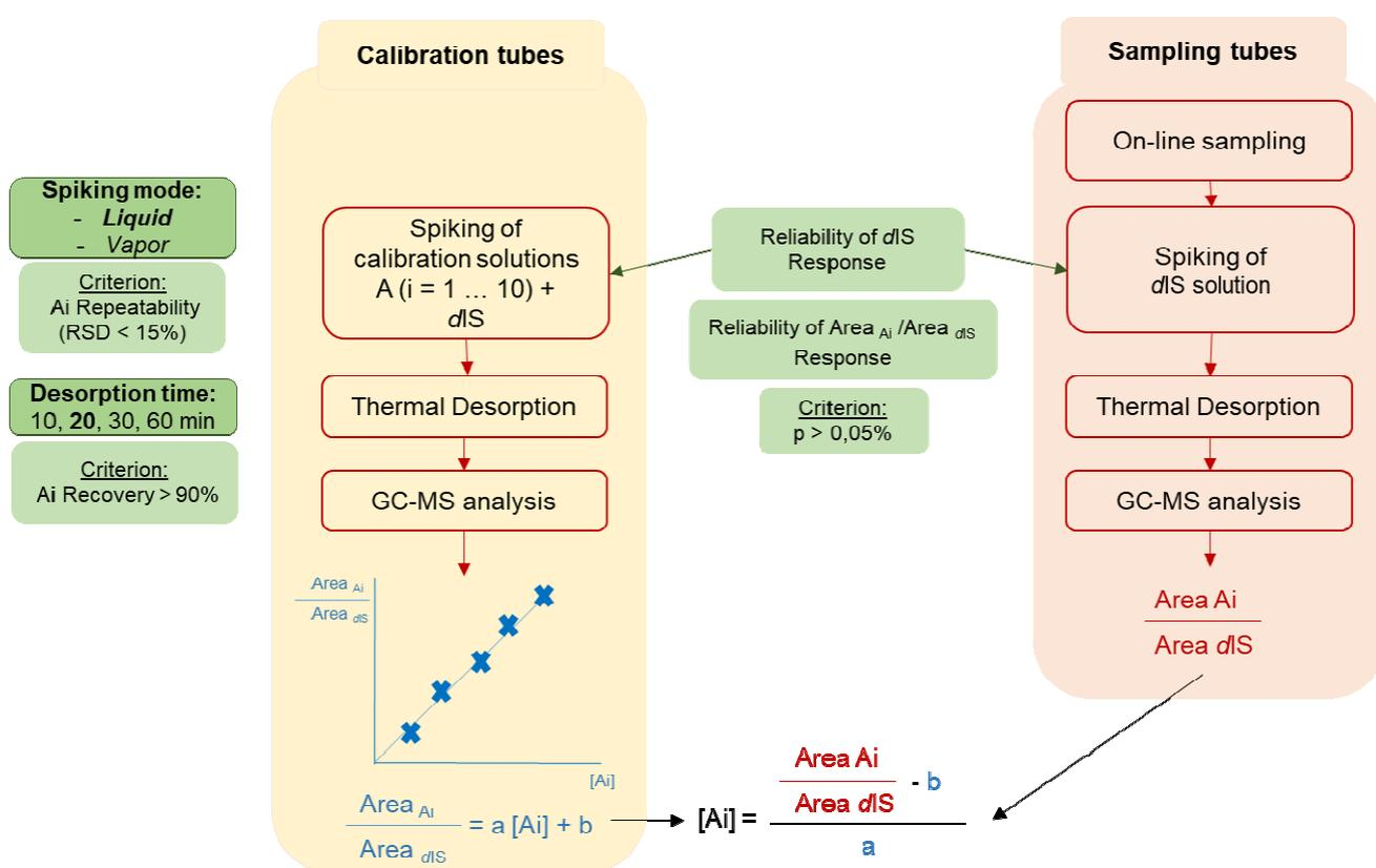
Figure 11 : Analytical strategy applied for the development and validation of the quantitative TD-GC/MS method: the analytical steps are circled in red while the parameters tested are in dark green and the performance criteria chosen for the optimization are in light green. Publication in progress.
