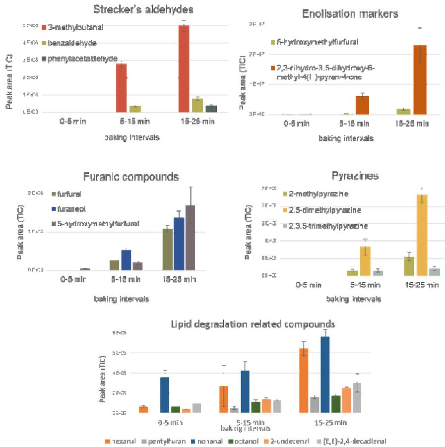
Figure 16: CNFV monitoring during baking by dynamic SPME extraction. Based on (ACL14).
