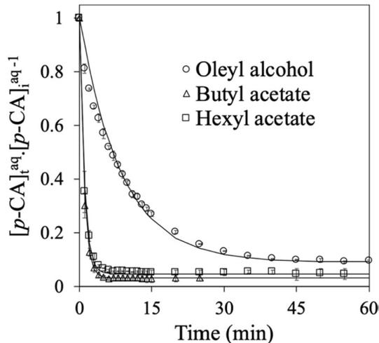
**Fig. 3.** Kinetics of *p*-CA extraction from binary solution pH 3.7 with the studied solvents. Lines correspond to equation (4) for aqueous content of *p*-CA with respective  $\tau$  (Table 3).
