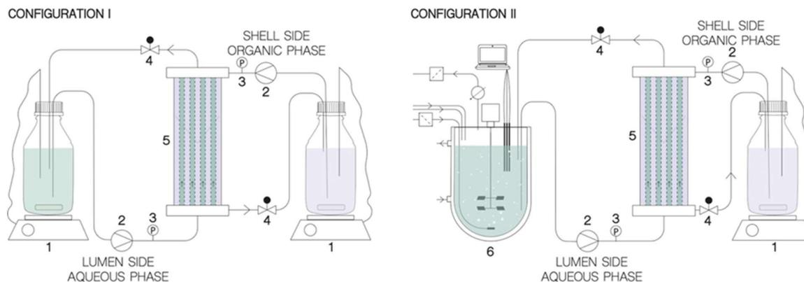
**Fig. 1.** Schematic experimental setup diagrams. Configuration I: Experiments with model solutions; Configuration II: Final coupling experiment with real fermentation; 1: stirring and heating plate; 2: pump; 3: manometer; 4: pressure valve; 5: HFMC; 6: controlled bioreactor.
