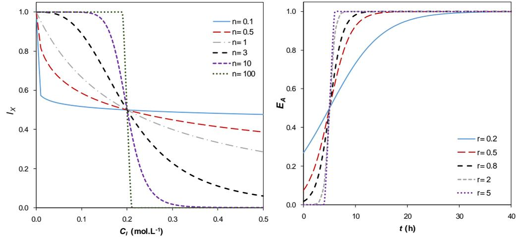
**Figure 3.** (a) Example of inhibition factor  $I_X$  as a function of  $C_I$  for different  $n$  values and  $K_{IX} = 0.2$  mol L<sup>-1</sup>. (b) Example of enzymatic activation factor  $E_A$  as a function of  $t$  for different  $r$  values, and  $t_{lag} = 5$  h.
