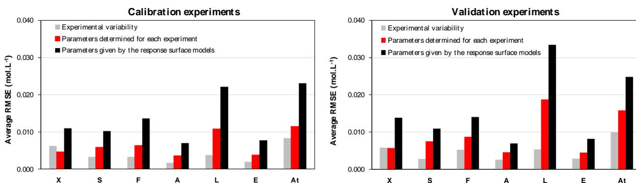
**Figure 7.** Comparison between experimental variability and average RMSE values for concentrations computed using parameters determined for each experiment (Table 2) and the response surface models (Table A2 and Equation (17)).
