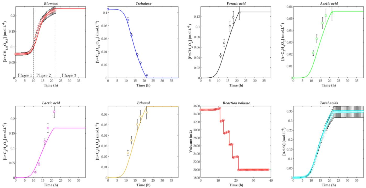
**Figure 5.** Evolution of concentrations over time for experiment F10 ( $T = 30\text{ }^{\circ}\text{C}$ ,  $\text{pH} = 8$ ). Comparison between model (continuous line, using parameters from Tables 1 and 2) and experimental data (symbols). The error bars for data represent the biological standard deviation, calculated from three independent repetitions of the run F01.
