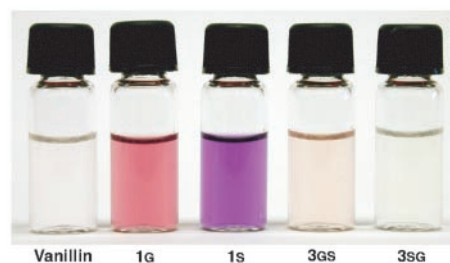
FIG. 7. Picture of freshly prepared phloroglucinol-HCl-treated solutions of the hydroxybenzyl aldehyde vanillin, hydroxycinnamyl aldehydes 1G and 1S , and two hydroxycinnamyl aldehyde 8-O-4-coupled models, 3GS and 3SG . The characteristic lignin staining is only achieved with the hydroxycinnamyl aldehydes 1 . UV spectra show that the characteristic peak at ~550 nm is not present in products from the hydroxycinnamyl aldehyde 8-O-4-coupled models 3 .
