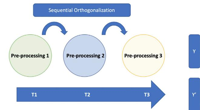
**Fig. 1.** An illustration of the SPORT approach for pre-processing fusion. SPORT involves sequential PLS and orthogonalization steps to extract scores from differently preprocessed data. Later all the scores are concatenated and used for ordinary regression analysis.
