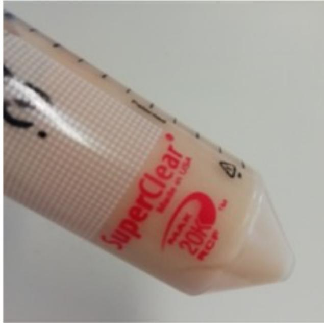
**Figure 7: Small decantation after 30 min at 3,000 rpm for E898**
