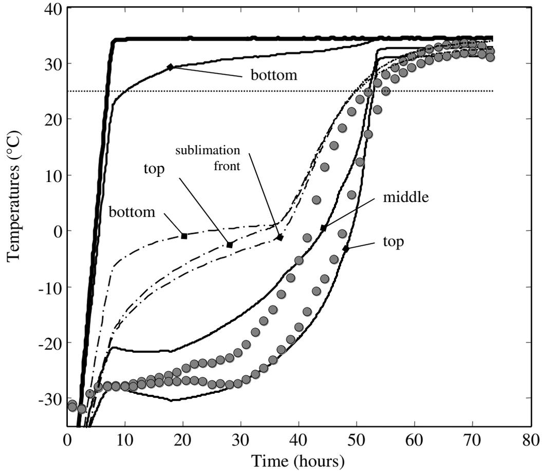
Figure 2. Model validation based on product temperature. Measured product temperature (symbols), product temperature calculated by the presented model (solid), product temperature calculated by a compact layer model (dash-dotted), shelf temperature (bold) and chamber temperature (dotted).
