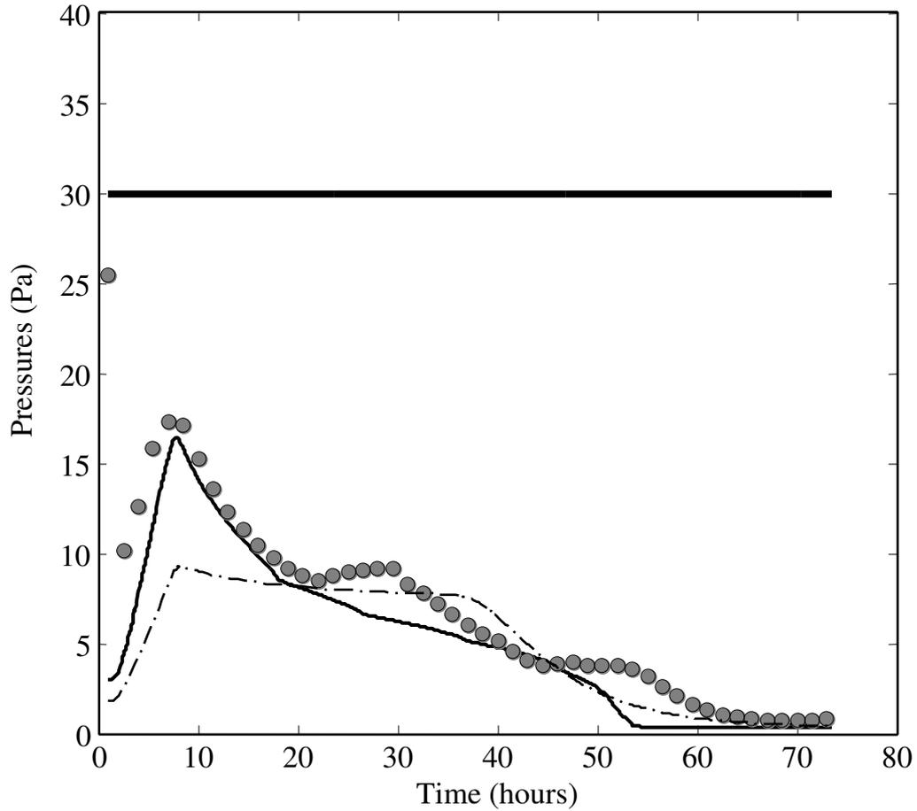
Figure 3. Model validation based on partial vapor pressure in the chamber. Measured vapor pressure (symbols), vapor pressure calculated by the presented model (solid), vapor pressure calculated by a compact layer model (dash-dotted), total (vapor + inert gas) pressure in the chamber (bold).
